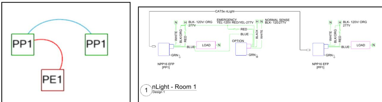
Figure 42 - Riser Diagram
