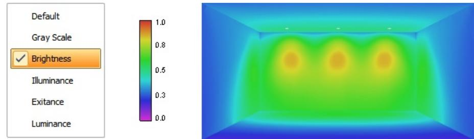
The **Illuminance** mode shows the **Rendering** with pseudocolor shading that maps *illuminance* onto all surfaces with actual calculated *illuminance* used for scaling.
