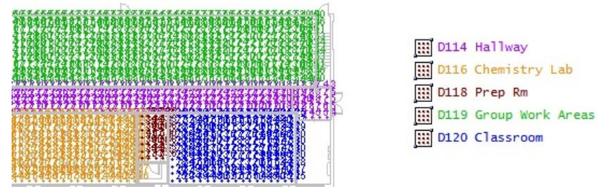
Point values can be highlighted based on an **Upper Limit** and/or a **Lower Limit**. To modify highlights, edit the **Calculation Zone Properties**, and make **Color** and/or **Value** selections as desired.
