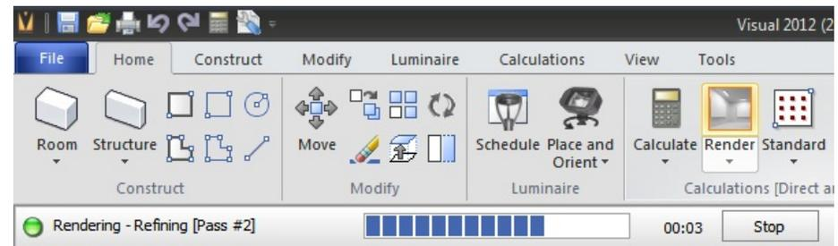
**Luminaires** are displayed in a **Rendering** as defined in the [Model tab](#) of the [Luminaire Editor](#). If a [Luminaire Model](#) is not defined, the **Luminaire Symbol** will be used.
