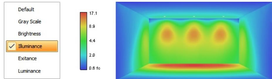
The **Exitance** mode shows the **Rendering** with pseudocolor shading that maps the *exitance* off all surfaces. Note that [Exitance](#) factors *illuminance* by the **Reflectance** of the base **Solid Object**.
